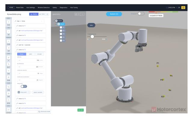
Motorcortex-Robot-App is a turn-key motion control software for multi-axes Serial and Parallel Robots. It provides the machine logic, kinematics, motion control, errorhandling and interfacing to hardware. Shorten your time-to-market and reduce software development time
